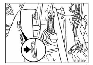
Take off locking clip for shaft pin of clutch-sensor cylinder.
