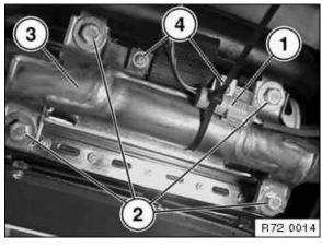
If necessary, unfasten cable tie for plug connection on airbag module. Open lock on connector (1) by applying pressure to tab and unfasten the connector.
