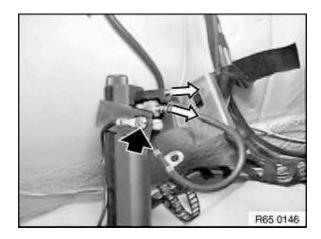
Loosen screws, pull off connector and remove antenna from bracket.
