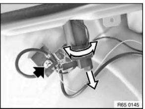
Unfasten nut and pull antenna downward out of rubber grommet by twisting back and forth.
