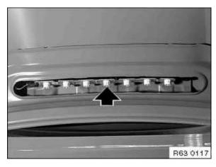
Twist the defective lamp socket and remove. Light bulb out of socket
