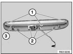
Release screws (1) and remove brake light (3).
