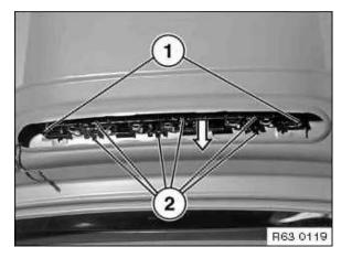
Unscrew bolts (1). Unclip frame at clips (2). Lift lamp glass up to remove.
