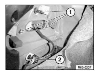
Unscrew nuts (1). Disconnect plug connection (2) and pull out rear light.
