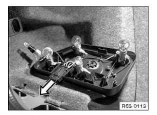
Remove connector and fit light bulb.
