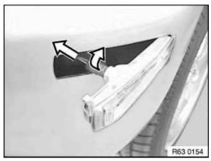
Turn lamp socket by approx. 90  $^{\circ}$  and pull out.
