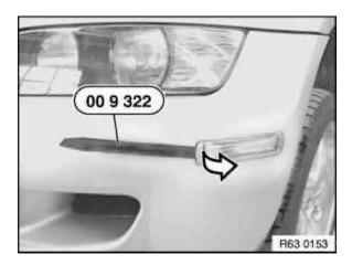
Lever out side-marker lights at front with special tool 00 9 322 (plastic wedge).
