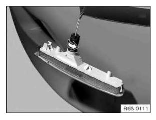
Twist lamp socket and lift out.
