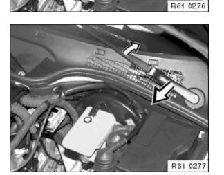
Unscrew left and right nuts. Tightening torque, 61 61 10AZ
