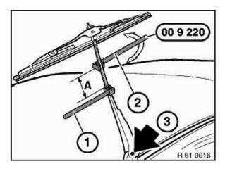
If the contact angle is incorrect, the wiper arm must be turned into correct position using two special tools 00 9 220.
