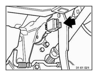
Brake-light-test switch is in same housing as brake-light switch. For removal and adjustment, refer to brake-light switch 61 31 310. Can be recognized on 4-pin connector.
