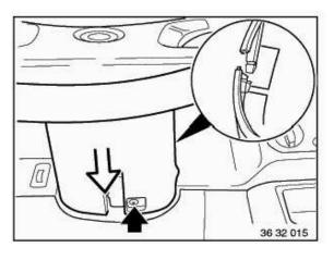
Remove screw and take off lower section of steering-column panelling.
