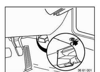
Turn steering wheel to straight-ahead position. Remove steering wheel, refer to 32 33 000 Remove instrument panelling at bottom left.
