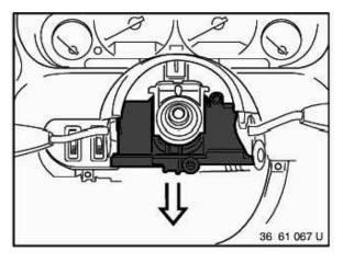
Lever off holder in downwards direction using a screwdriver.
