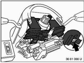
Remove screw for holder of steering-column stalk.
