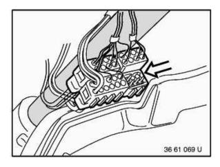
Loosen cable straps on steering column.
