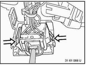
Compress retainers on both sides and pull out lever.
