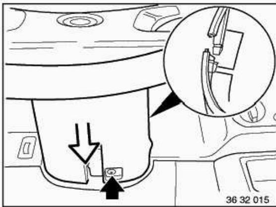
Remove screw and take off lower section of steering-column panelling.
