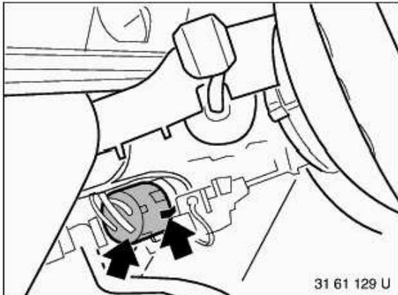
Unscrew headless screws on both sides, pull out switch.
