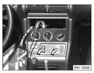
Remove radio finisher or, if necessary, radio, refer to 65 11 030 Push a/c switch or indicator lamp forwards through radio aperture to unclip and remove connector.
