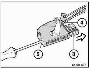
Press contact carrier (3) and cables out of aperture (5).
