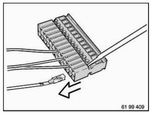
Hold down arrester hook once again in secondary lock (8) and pull cable and contact completely out of contact carrier.
