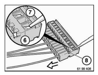
Hold down arrester hook (6) of defective contact and pull cable and contact up to secondary lock (8).
