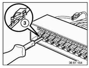
With special tool 61 1 136 or 61 1 137 (ejector), press back arrester hook (3) of appropriate contact and pull out cable.
