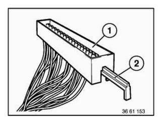
Pull relevant fuse out of fuse block (1).
