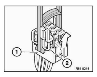
Place special tool 61 1 153 on relay carrier (1) and carefully pull in direction of arrow until retaining lugs (2) on relay carrier are raised.
