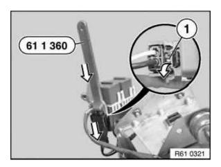
Unlock hook (1) with special tool 61 1 360 and slide plug housing downwards out of base.
