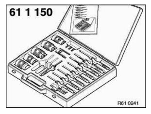
Special tool 61 1 150 (release and pressing-out tool) for:
