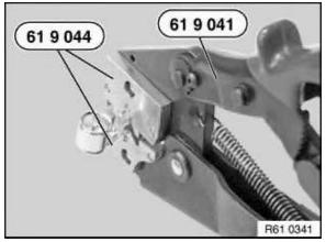
Special tool 61 9 041 (hand pliers) with special tool 61 9 044 (matrix) for crimping cable guide and strain relief device on antenna elbow plug.
