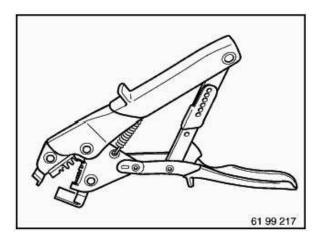
Special tool 61 9 041 (hand pliers) with special tool 61 9 042 (matrix) for crimping connectors and contact tubes for fan connectors up to a wire cross-section of 2.5 mm <sup>2</sup> and for pushing on contact tubes for fan connectors.
