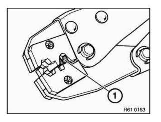
Preload contact by squeezing matrix in crimping tool. Grip contact (1) firmly only, do not crimp.
