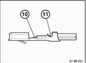
Correct crimping: Visible conductor end (10). Visible insulation end (11).
