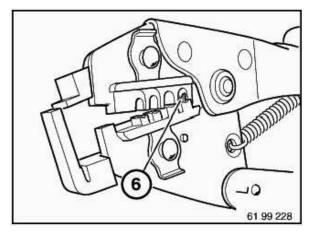
Preload contact by squeezing matrix in crimping tool. Grip contact (6) firmly only, do not crimp.
