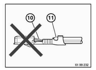
Incorrect crimping: Conductor end (10) inserted too far. Insulation end (11) in wire crimp. If necessary, repeat crimping with a new contact.
