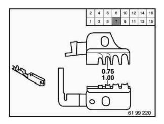
Contact sleeve for fan connector
