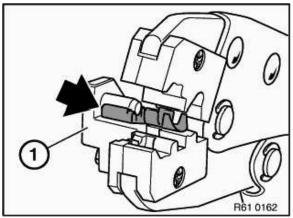
Insert contact sleeve  $4 \text{ mm}^2$  in nest with lock (1) as far as it will go.
