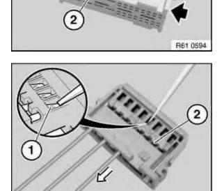
Hold down retaining hook (1) of socket contact in opening of contact carrier with a small screwdriver.
