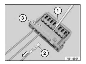
Hold down retaining hook in secondary lock (1) again and pull cable with socket contact (2) completely out of contact carrier (3).
