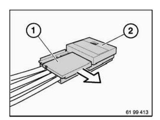
Pull connector (1) (slide) off contact carrier (2).
