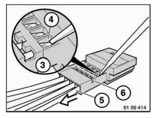
Hold down arrester hook (3) of defective contact and pull cable and contact up to secondary lock (6).
