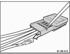
Hold down arrester hook once again in secondary lock and pull cable and contact completely out of contact carrier.
