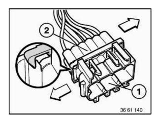
Move connector upper section (1) and connector lower section (2) against each other in direction of arrow.
