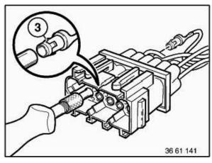
With special tool 61 1 132 (ejector), press back arrester hook (3) of appropriate contact and pull out cable.
