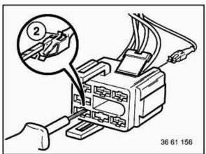
With special tool 61 1 136 or 61 1 137 (ejector), press back arrester hook (2) of appropriate contact and pull out cable.
