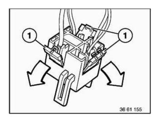
Unlock locking flap (1) of corresponding cable.
