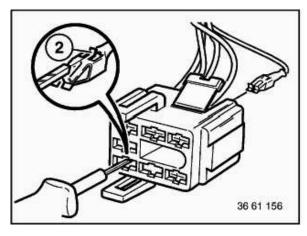
With special tool 61 1 136 or 61 1 137 (ejector), press back arrester hook (2) of appropriate contact and pull out cable.
