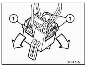
Unlock locking flap (1) of corresponding cable.
