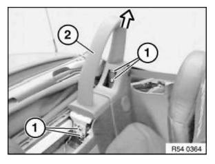
Version with "Harman-Kardon" Hifi system: Loosen screws (1) by 10 mm and pull out roll bar (2) upward.
