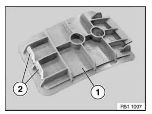
Version with "Harman-Kardon" Hifi system: Removing and installing loudspeaker box, refer to 65 13 300 Unclip cover (1) with long screwdriver through opening for seat belt.
