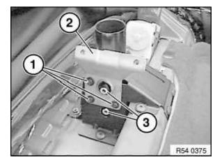
Version with Harman-Kardon Hifi system: Unfasten screws (1) and remove bracket (2). Replace screws (3).
