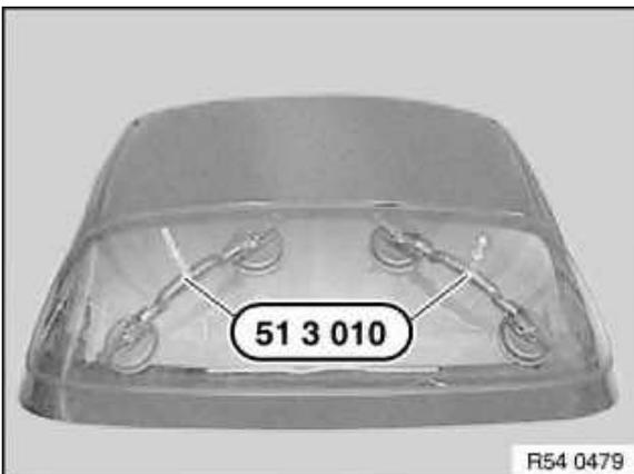
Install rear window carefully using special tool 51 3 010.
