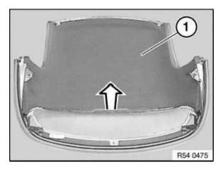
Raise molded roof lining (1) at rear window and slide towards front.
