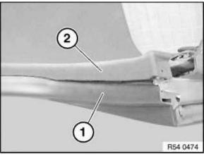
Pull off molded roof lining (2) from rubber seal at front (1) towards inside.
