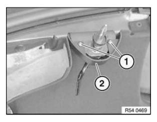
Release screws (1) and remove cover (2). Remove panel, rear window frame, bottom, refer to 54 21 090.
