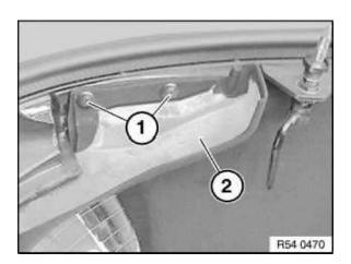
Release expansion rivets (1) and remove panel, rear window frame, bottom (2).
