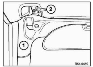
Release screws (2) and remove mounting plate.
