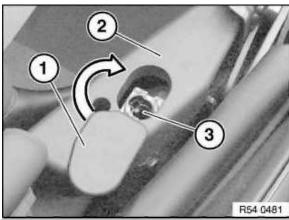
Close off hard top locating point (3) with cap (1) on cover at top of B-pillar (2).
