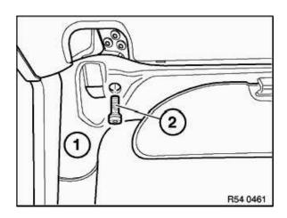
Release screws (2) on left and right in cowl panel (1).
