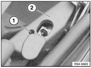
Unscrew bolt (1). Remove cover at top of B-pillar (2). Fit hard top and lock.
