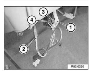
Disconnect plugs (1 and 2). Version with seat heating: Disconnect plugs (3) and (4). Lift out front seat.
