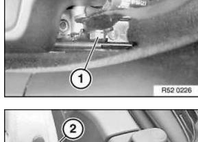
Withdraw seatbelt strap (1) from seatbelt guide (2).
