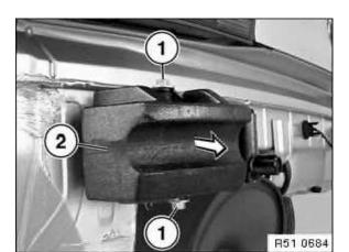
Loosen nut (1) and pull vibration damper (2) backwards to remove.
