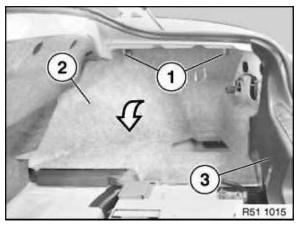
Version with battery in luggage compartment: Unfasten clips (1) and remove trunk wheel housing trim (2).
