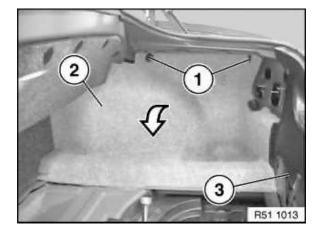
Version without battery in the luggage compartment: Unfasten clip (1) and remove trunk wheel housing trim (2).
