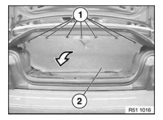
Version without Hifi system, without CD changer: Unfasten clips (1) and remove trim (2) for luggage compartment separating wall.
