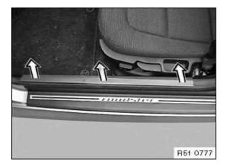
Pull rocker panel strip upwards to unclip.
