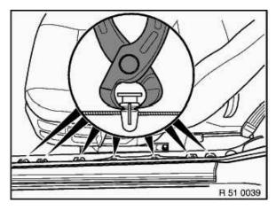
If necessary, squeeze clips together with pliers and lift out (head of pliers ground smooth).
