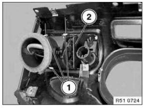
Lift off interlocks (1) and pull air vents (2) forwards to remove.
