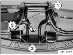
Unfasten screws (1) and metal tabs (2) and remove centre of air guide (3).
