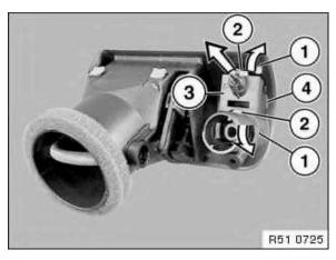
Press air vents (1) apart until the interlocks (2) are released and remove light insert (3).
