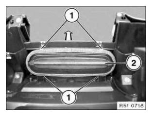
Lift out interlock (1) and pull out centre of air vent (2).
