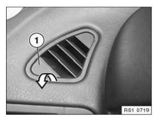
Pull left/right air vent (1) downwards (with feeler gauge) and remove.
