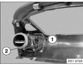
Lift off interlocks (1) and remove air vents (2).
