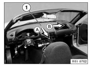
Lift instrument panel (1) upwards and backwards (A) and remove on passenger side (B).
