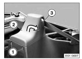
Remove caps (1) and screws. Pull out upper section of side trim panel (2) upward/forward over the seat belt roller (3).
