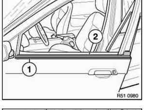
Using special tool 00 9 311, starting at back, (1) and moving to front (2), lift out window cavity cover strip.
