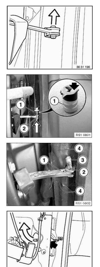
Old build status: Drive rivet out in upwards direction. Pull off rubber grommet.
