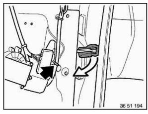
Slide rubber grommet to one side and, if necessary, unfasten cable strap.
