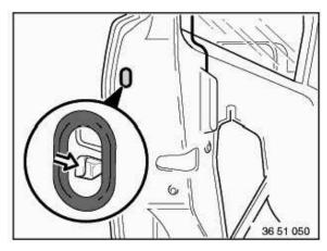
Push slide forwards with special tool 51 3 190 and remove finisher from outside handle.
