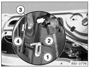
Unclip retainer (1) and lift out linkage (2). Press outside handle (3) slightly down, disconnect from gate on door lock (4) and remove.
