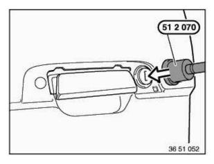
Unscrew nut using special tool 51 2 070 and take off outside handle.
