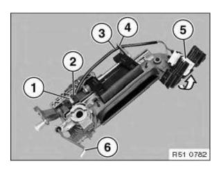
Remove clip (1) and lift out micro-switch (2). Remove cable (3) from the guide (4). Twist contactor socket (5) and remove. Remove actuating rod (6).
