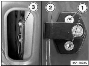
Unfasten screws (1) then remove threaded plate (2) and striker (3)
