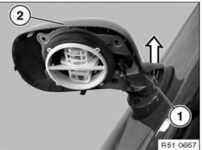
Carefully slide guide (1) forwards (risk of damage) and remove rear section of housing (2).
