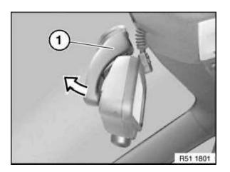
Snap mirror (1) forwards out of mirror mount and remove.
