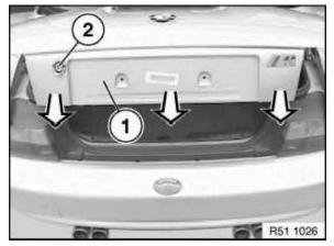
Pull off rear trim panel (1) all around, lift over lock cylinder (2) and remove towards rear.
