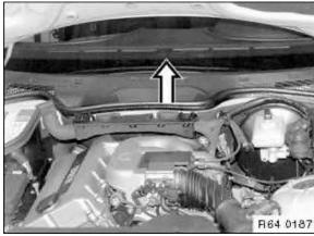
Unfasten all expanding rivets and remove protective grill.
